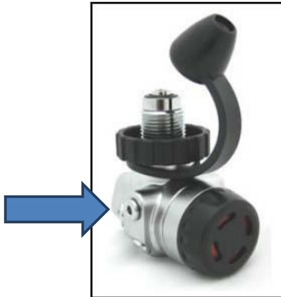
Check that the threads on the plug match in size and number to the threaded fitting of the LP hose. If the thread on the regulator port is different, an adapter plug will be required. Clean the O-ring on the threaded end of the LP Hose then screw the threaded fitting into the regulator port. Use a wrench to snugly tighten the threaded fitting. Do not over-tighten.
